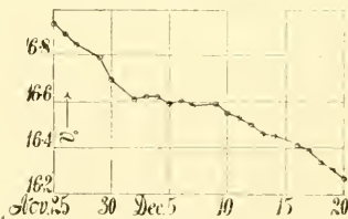
FIG. 24.—Chart showing loss of standard volumes of gas in diver in lapse of days. Diffusion of air through KCl solution.
